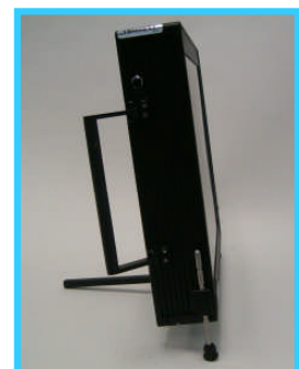
Thin profile with retractable legs and fold-out stand provides convenience and portability.
