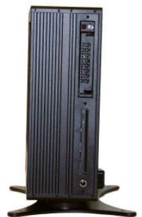
Side View showing Removable Hard Drive and DVD/CD-R Drive Bays
